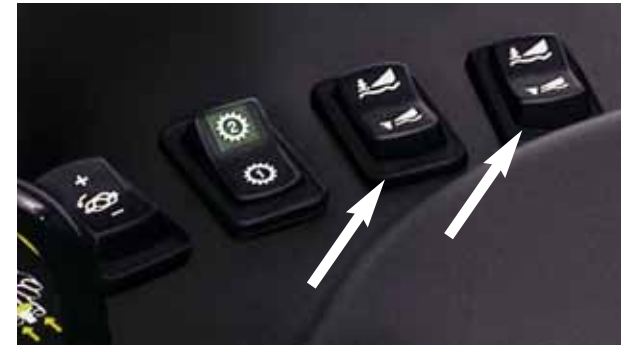
Dual switches in the WD1903 and WD2303 cab allow you to control the flotation of the left and right side of the header independently.
