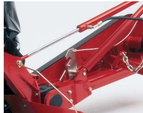
Adjustable flotation spring(s) allow you to change the ground pressure applied to the MDX cutter bar.
