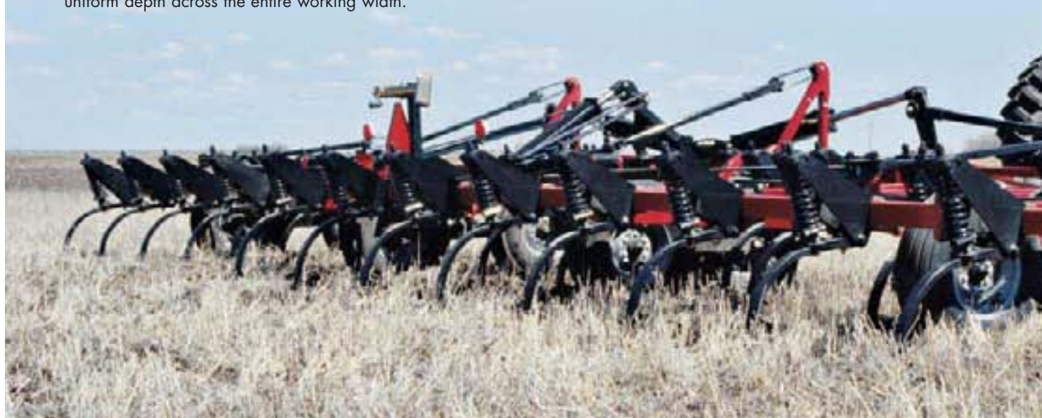
550 or 650 lb. (250 or 295 kg) trips are available to match field conditions.
