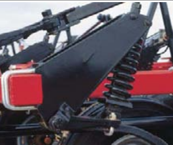
550 or 650 lb. (250 or 295 kg) trips are available to match field conditions.
