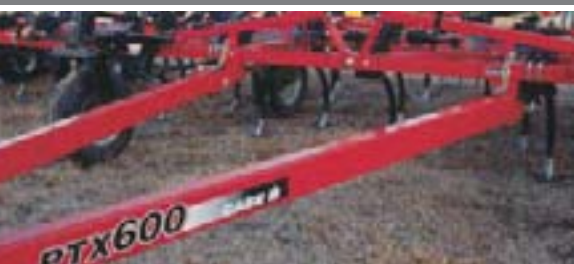
Floating hitch provides improved front-to-back land following capabilities.
