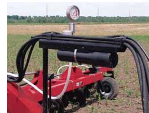
The front hose stand keeps hoses and wires away from the tractor hitch.
