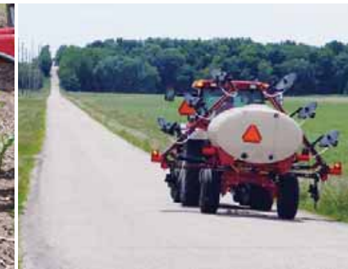
Wings fold over center for safe and convenient transport when moving from field to field.
