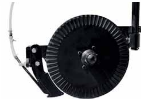
The cast chromium carbide 1/4 in. knife assures that all liquid fertilizer is applied at knife depth. Minimum 10 PSI is recommended.
