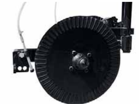
The liquid injector directs a high-pressure stream of liquid fertilizer into the coulters slot. Liquid injectors are very low maintenance. 40-100 PSI is recommended for precise application.
