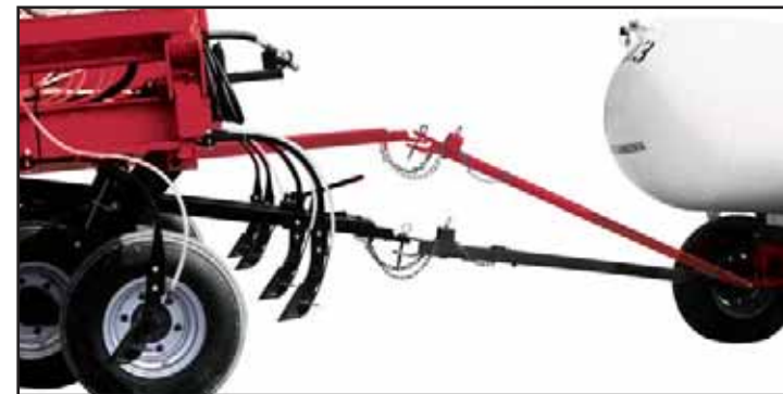
Case IH Wagon-Mate™, Constant-Tongue-Height Hitch With its simple, trouble-free mechanism, the hitch protects tongues from damage, keeps the wagon tongue level when applicator is in raised or lowered position and is designed for easy viewing of the wagon hitch when backing up to nurse tanks.
