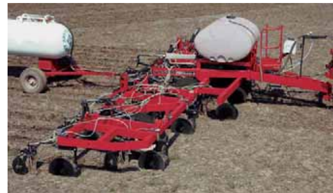
500-gallon liquid tank optional for dual-placement capability, available on Pull-type models.
