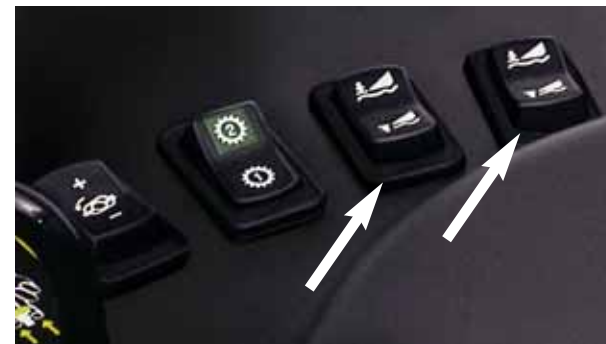
Dual switches in the WD1903 and WD2303 cab allow you to control the flotation of the left and right side of the header independently.
