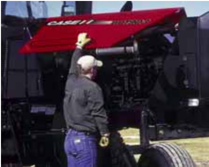
Side shields flip up for easy access to the engine. From ground level, you easily can reach all key maintenance points, including fluid levels and filters. You'll spend less time servicing your windrower, more time out in the field producing!
