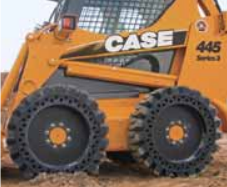
▲ Whatever the application, Case has a tire to fit your needs. For example, SolidFlex tires (shown here) are a good choice to avoid the downtime associated with flat tires.
