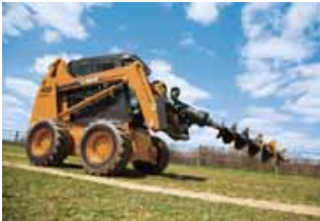
▲ The two speed drive motors (standard on 450 and 465, optional on all other models) make faster travel speeds possible, when moving material around the farm or when roading between fields.
