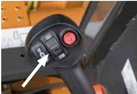
▲ The thumb-operated, proportional, auxiliary control option puts precise and easy control of the attachment right at your finger tips.
