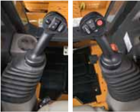
▲ The standard, low-effort, servo-hydrostatic controls provide precision operation for greater productivity. Optional pilot controls have a shorter lever throw and require even less effort than the standard controls, resulting in more precise operation and less wear and tear on the operator over the course of the work day.
