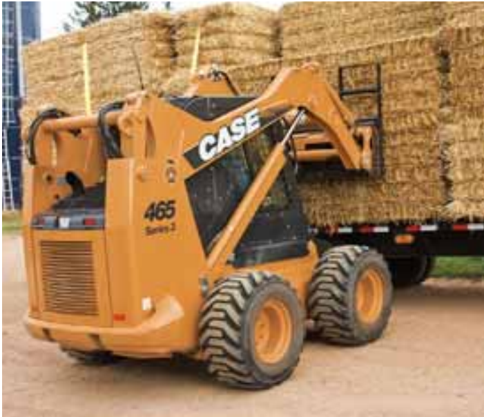
▲ The Power Reach , vertical lift, loader linkage provides maximum reach at any height, making it easy to place material on trailers and load into the middle of high-sided trucks.
